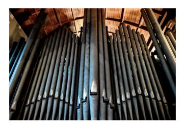
In 2014, Nicholson & Co. carried out a complete refurbishment of the instrument. All of the original action was stripped out and replaced by a modern 'exhaust' electro-pneumatic system, and the pipework was cleaned and restored.
